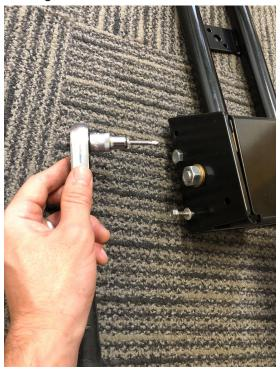
STEP 2: Once fixings are removed - lift out the spring cover.
