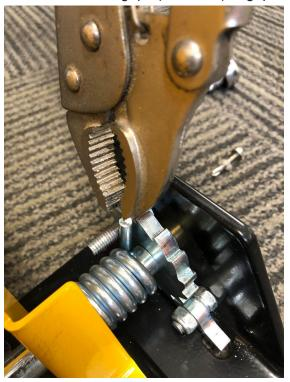
STEP 4: Apply pressure by pulling back the spring whilst turning the gear cog in the same direction and set the locating pin in the next slot on the cog.
