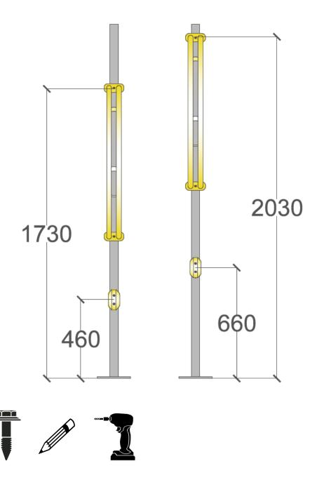
To secure the Cradle to the post, lay the Silver Bullet on the protected floor. Using the measurements listed above, mark the top fixing holes on the post. Secure the cradle to the post by using self tapping screws and an impact driver, be careful not to overtighten. Once you have secured through the top fixing hole, do the same for the bottom. Using the heights listed above, secure the wheel catchers to the post, again with self tapping screws.
