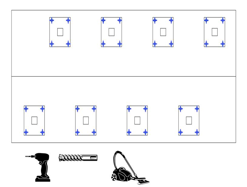
On each base plate of the Silver Bullet, there are four fixing points. Using a 10mm SDS drill bit, drill all of the points (indicated with a +). Once you have drilled all the holes, vacuum up the dust.
