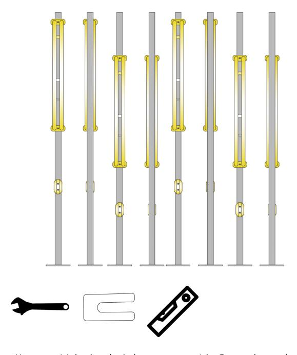
Use your spirit level to check the posts are straight. For any that need adjustment, loosen the bolts and insert a window packer under the baseplate of the post. Once the posts have been levelled, the installation of the Silver Bullet is complete.
